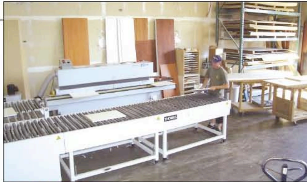
Return on investment — Shop owner David Wilhoite added this Thomas Machinery return conveyor to his Brandt edgebander so one operator could be more efficient. Now edgebanding and CNC work continue simultaneously with one worker.
