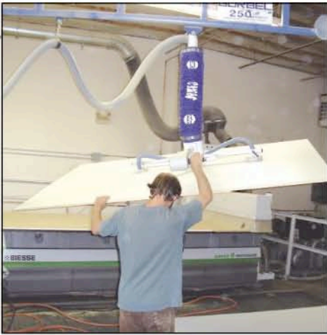
Up, up and away — Adding a Schmalz vacuum lift made it faster and safer for workers to move sheet materials
